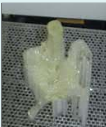
FIGURE 7. A LASER BEAM SWEEPS LAYER-BY-LAYER USING A UV LIGHT TO CREATE THE BIOMODEL. THIS DEPICTS THE HEAD OF A FEMUR.
